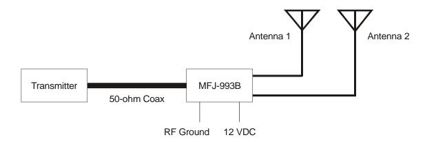
Figure 1. Installation Block Diagram.
